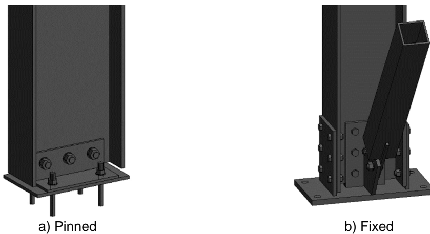
Fig. 4.8 Examples of demountable base connections to columns
