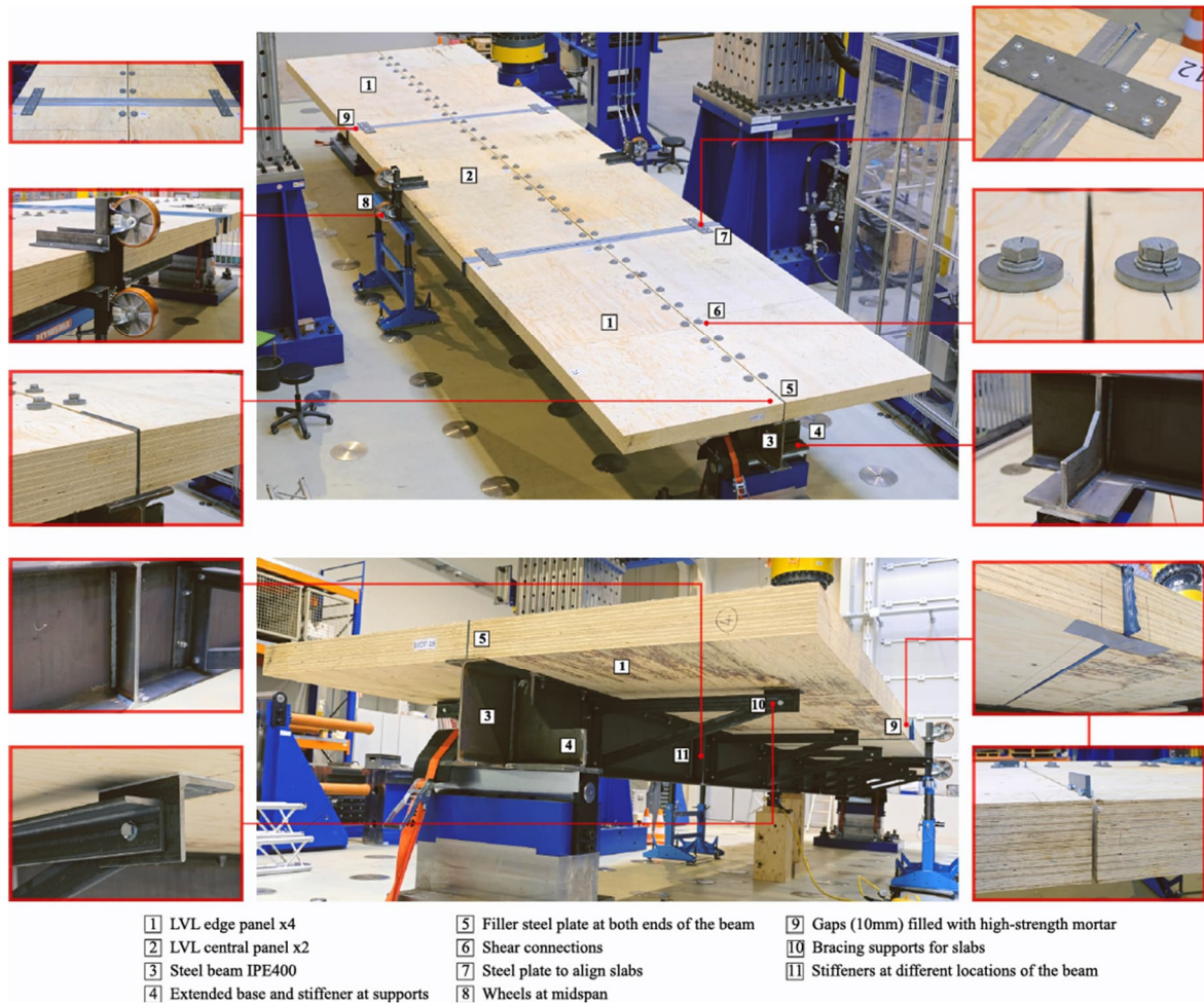
Fig. 4.33 Components of the SCT beam specimens [49]
