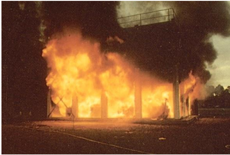
Figure 5: Test structure at BHP Melbourne Laboratory Australia simulating the 41-storey office at William St.
