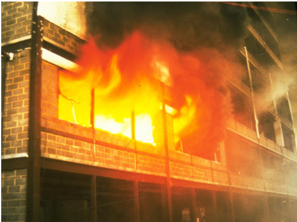
Figure 1: Fire test of an office in the 8-storey Cardington building. The temperature reached over 1200°C and large volumes of dense smoke were generated.
